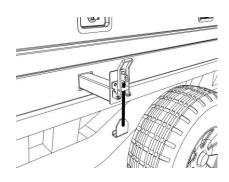
**Step 1**. Align the Ridgeback service body on the vehicle tray between 30mm to 50mm from the cabin/headboard.
