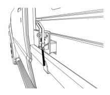
**Step 3**. Hook each clamp under the tray and align the toggle latch vertical with the tray side
